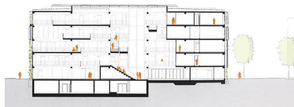
The design of the floor plan changes in every storey and thus provides a lively circulation.
